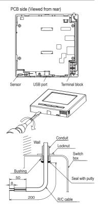
② When wires are passed through the bottom case, fix the bottom case at 2 places on the switch box.
