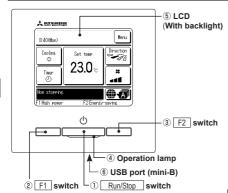
Touch panel system, which is operated by tapping the LCD screen with a finger, is employed for any operations other than the ① Run/Stop, ② F1 ③ F2 switches.
