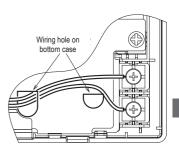
When taking the wiring out from the upper center, open a hole before separating the upper and bottom cases. This will reduce risk of damaging the PCB and facilitate subsequent work.
